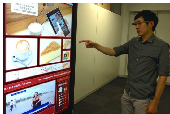
Figure 1. We report our approach to realize contents transfer from multi-section digital signage to users' private device, such as glass-like system and smartphones. We use computer vision approach, which includes corner and line segment detection to identify signage layout within user's camera view.
